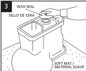
3 Put the toilet on a soft mat (prevent the surface of the toilet scratching). Take the new wax ring to be sure that it fits over the floor flange and fix it. Also check the sewer whether is
