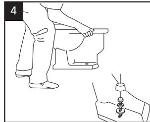
4 Carefully align the toilet to the hole on floor, adjust toilet until balance. Fix toilet by installing expansion bolts through toilet screw holes. Mildew proof silicon need to
