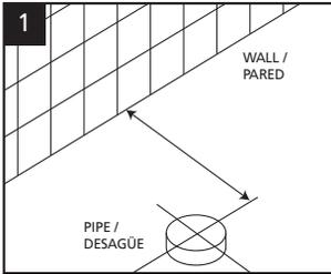
1 Make sure the floor drain pipe hole center, remark cross on the floor to be sure that aligning the toilet outlet hole to floor drain pipe.
