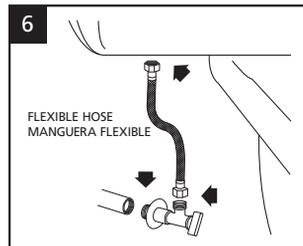
6 Connect the sink water inlet piping to the inlet angle valve.
