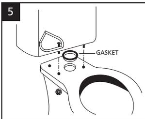
5 Install the gasket, then place tank over bowl and fix it with washers and nuts.
