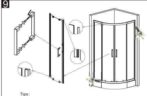
Allow the silicone to fully dry before operating the door suggest after 24 hours.
