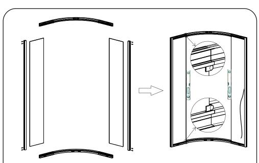
After assembly the alu. frame, check each parts to insure in good parallelism and perpendicularity.
